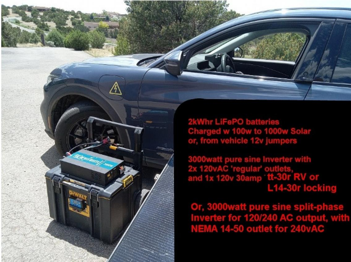
This system is enough for job sites, small cabin weekends, camping, charging cordless tools, and small 240v loads (like a shallow well with a small pump) if upgraded to the split-phase Inverter.
